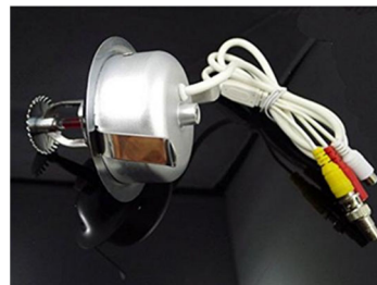
A CCTV camera that is installed inside a shell that resembles a sprinkler head
