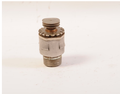
Recalled Omega Sprinkler Head
