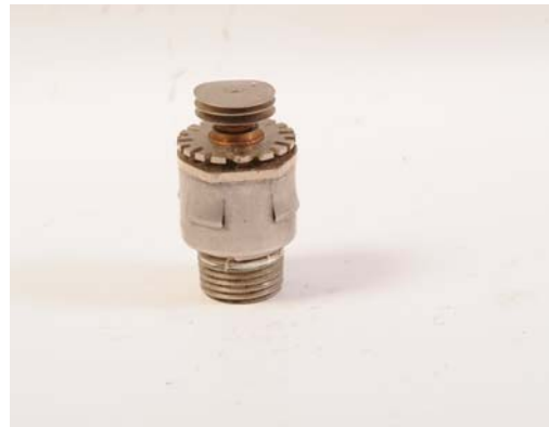
Recalled Omega Sprinkler Head
