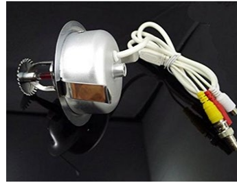
A CCTV camera that is installed inside a shell that resembles a sprinkler head
